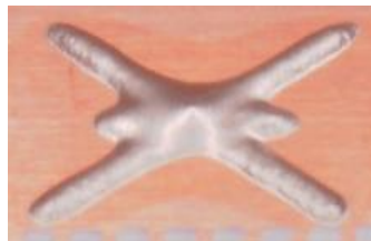
Dispense Patterns Visible solvent bleed out
